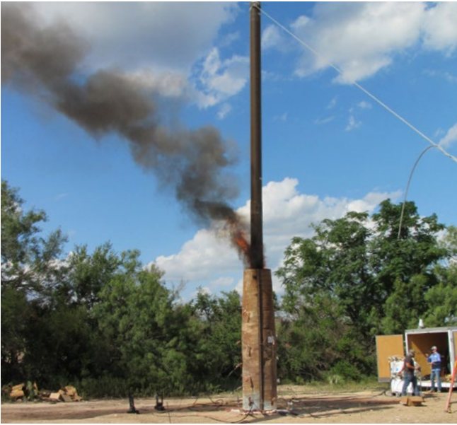
Fire Resistant Pole System being tested.
