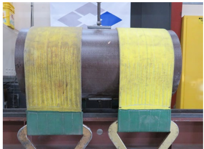
Bolt Pull Through Testing at EDM International
